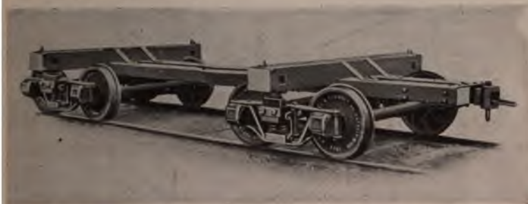
FIG. 89.—A Skeleton Log Car. A type common in the southern pine forests.
